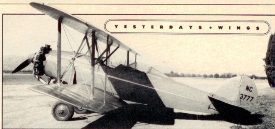
The first re-engined version of the Waco 10 on the market was the 1928 Model 125, powered with the 125-hp Ryan-Siemens SH-12 air-cooled radial engine imported from Germany.
