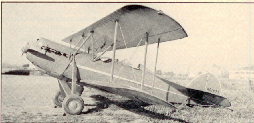
A popular engine change was the 115-hp Milwaukee-Tank air-cooled rebuild of the OX-5. This was called the GEX Special (above). A CTO Taperwing (below), cleaned up for racing, has the 240-hp Wright J-6-7 engine, low-drag landing gear and I-struts replacing the parallel struts.
