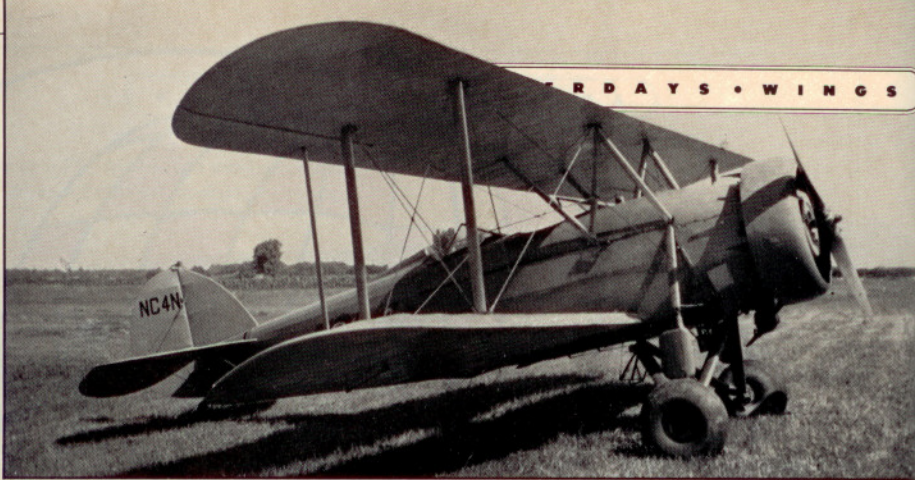
When the Packard engine of the HSO was replaced with the 220-hp Wright J-5 in the early 1930s, it became the ASO, shown above. In 1948 a change to a 220-hp Continental R-670 made it an ASO Special.
